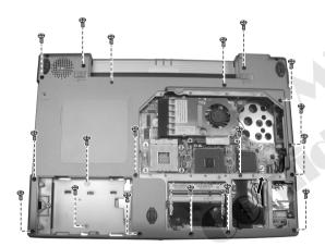
Figure 2-14 Remove the eighteen screws and separate the antenna
